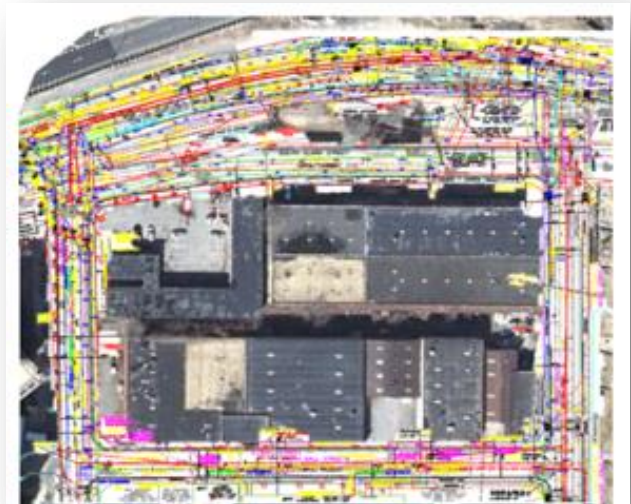
Figure 3 – Original Site with Existing Utility Overlay Courtesy of Davis and Google Maps
